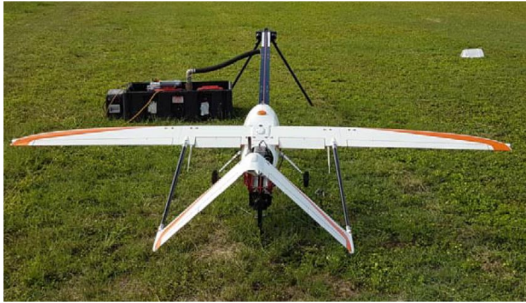
Survey RPA - Callsign Unmanned Laser – 3 metre wingspan, cruise speed 45 kts
