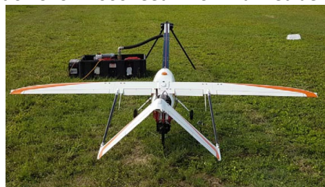
Callsign Unmanned Laser - 3 metre wingspan, cruise speed approximately 45 knots
