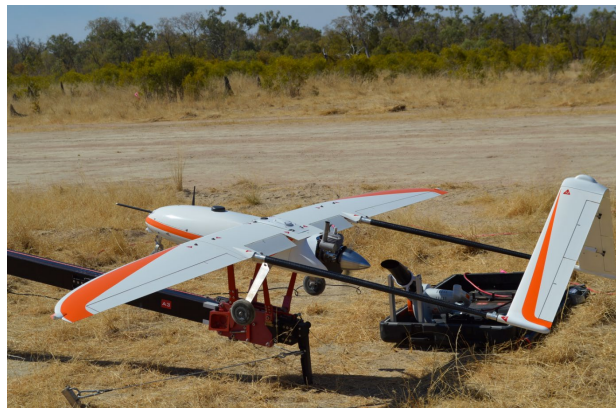
Callsign Unmanned Laser - 3 metre wingspan, cruise speed approximately 45 knots
